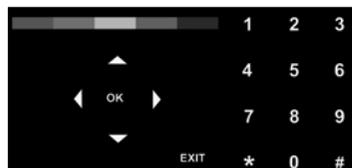
Navigate the menu tree via the Up/Down Directional buttons. When a menu is highlighted, open by pressing the OK button.
