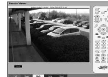
Navigation is via a colour coded softkey system. The colour bar menu provides an intuitive approach to operator and installer alike. The coloured buttons on the IR Remote Control and front panel correspond to the menu options displayed on screen.
